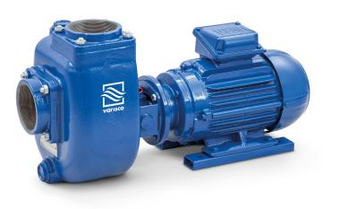
**Product Data** Suction port Threaded - 3" ISO 228 (BSP) Delivery port Threaded - 3" ISO 228 (BSP) Qmax 75 m<sup>3</sup>/h - 1250 l/min (330 USgpm) Hmax 20 m (65 ft) Solids handling 25 mm (1") Motor power 4 kW - 5.5 HP Motor type **IEC** standard Winding for inverters **Cast iron frame** Motor brand WEG W22 Premium Weight 65 kg (143 lb)
